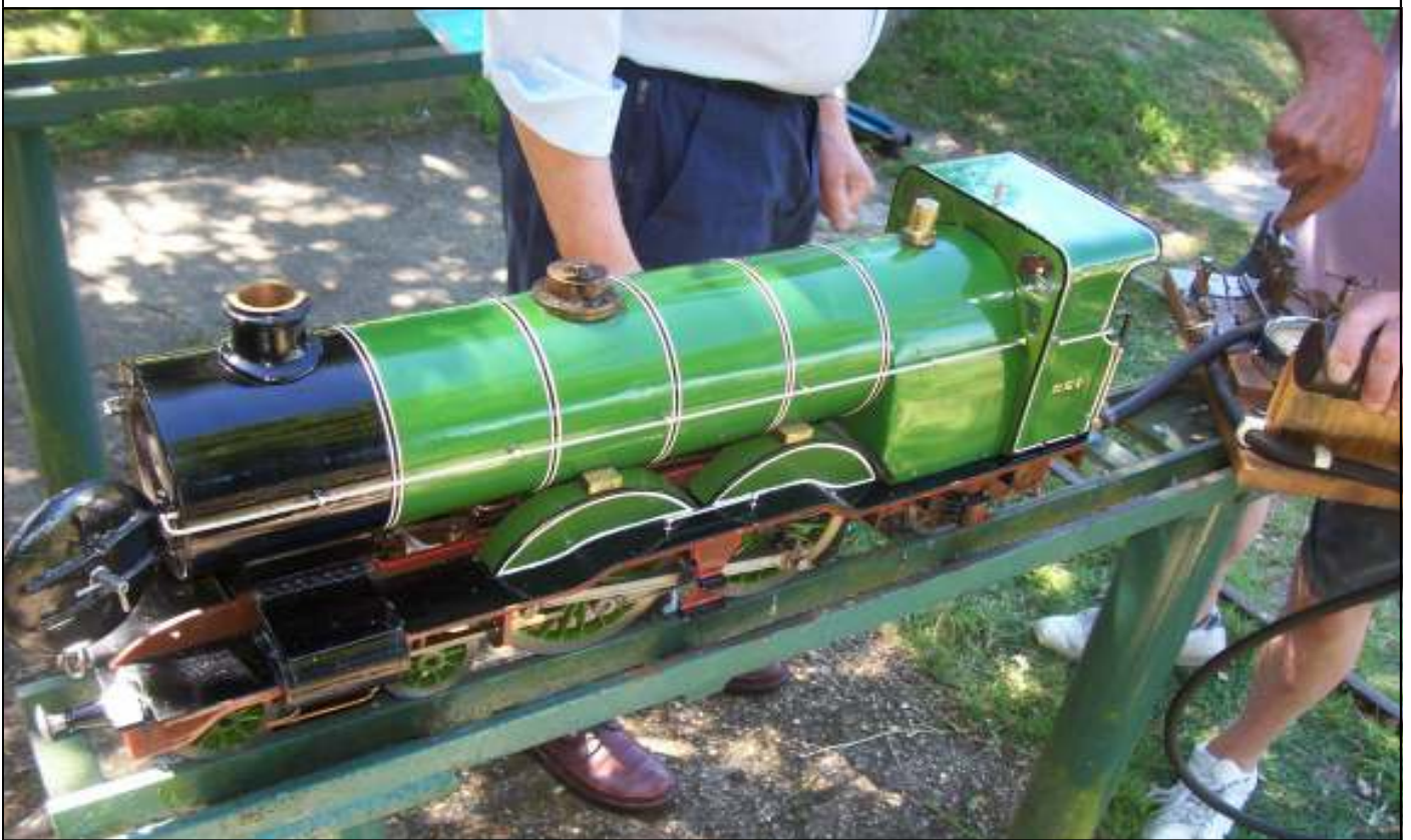
A view of Harry's Masie undergoing a 4 year hydraulic test, the safety valve has been removed blanked off. The test was completed successfully a the loco went on to pass it's steam test. The loco than ran most of the afternoon. GE 07/10
