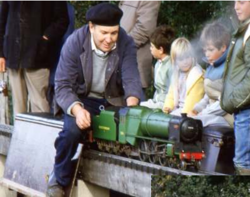
Robbie Archer driving a 3.5" gauge loco believed to be a variation on the 4-6-2 Hielan Lassie design by LBSC.
