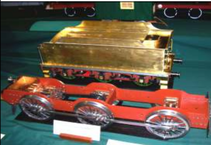
Another Don Young design a 5" Gauge POM POM . The photo does not do justice to the quality of the work which has been carried by Roy Gunn.
