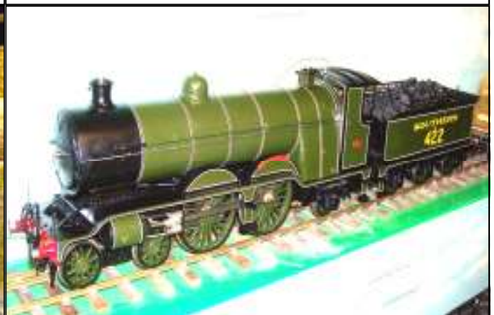
From the Sutton MEC stand; a fine example of a London Brighton South Coast 4-4-2 Atlantic, "North Foreland" finished in Southern Railway livery. The G1 loco is coal fired and to the Barrett Engineering design. Photos by D Newman and G Evans 04/09
