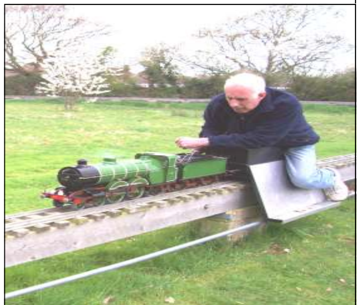
Dave Newman driving Harry Parry's 3.5 gauge Mona and testing the axle pump operation. Harry's Mona is also fitted with an injector which worked perfectly. Harry hopes to be attending the Romney Marsh MES open weekend with Mona. GE 04/09
